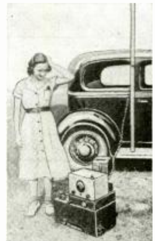
Photo at left shows author tuning 5-meter receiver of the portable automobile station used in the mountain-top tests made on the famous Skyline Drive in Va. Photo below shows young lady inspecting the 5-meter portable set; dynamotor and filter in bottom case, modulator in center case, and receiver on top.
