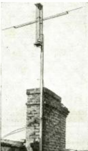
The 5-meter antenna and "L.L." oscillator erected on a chimney.
