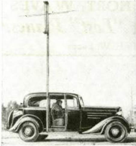
The 5-meter antenna and "Long-lines" oscillator atop pole, as used for portable station atop the Blue Ridge Mts., 3,600 feet above sea-level. The mast is lashed to the car so that the whole station is mobile.
