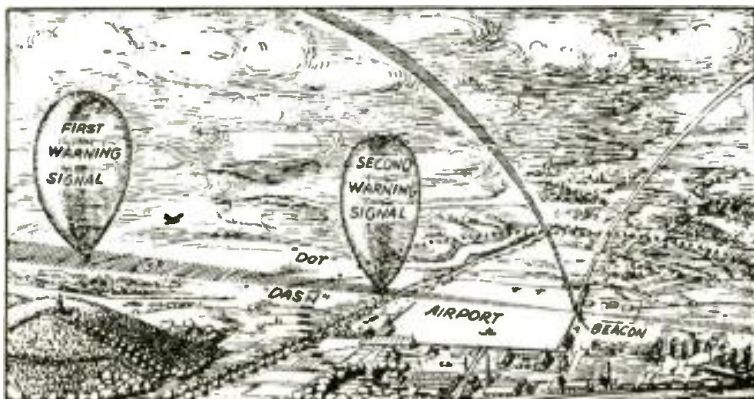
Above—a simplified drawing showing the effect of the first radio warning signal, second signal and also the radio guide beacon.
